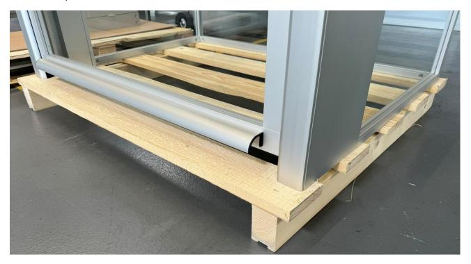
Since the roof surfaces are only placed in the insertion profiles, the enclosure is pressed over the roof onto the EU pallet or crate by means of polystyrene panels. Alternatively, they can also be fixed with a blue foam. This ensures that the roof surfaces cannot pop out during transport. Below is an example:
