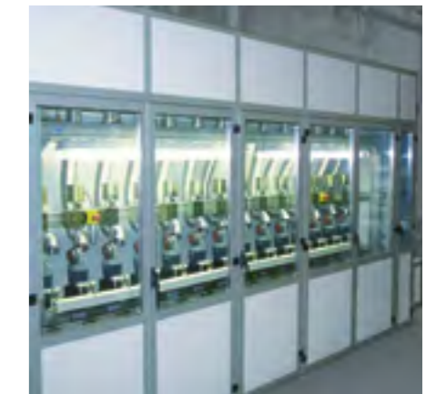
Protective cabinet and noise protection
